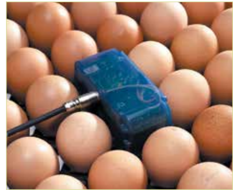
▲ OvoScan™ sensor positioned in an egg tray
